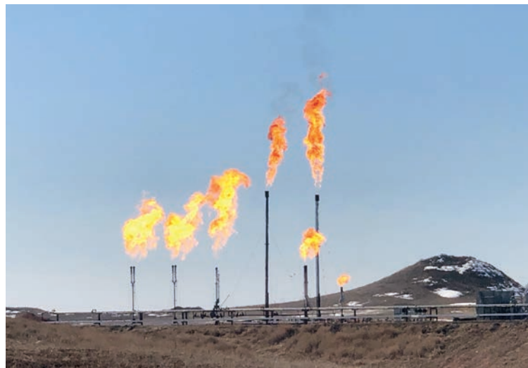
Oil drillers burn off the methane via flaring, which converts approximately 91.1% of the methane to CO 2
